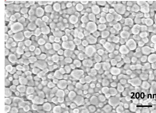
850 mW laser sintered line
